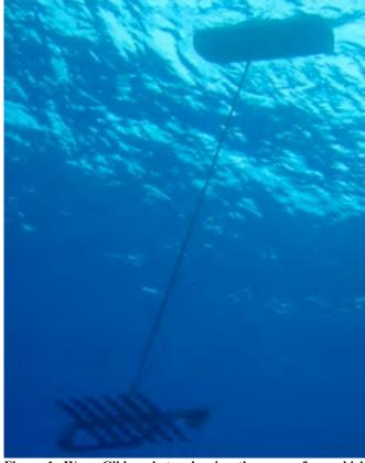
Figure 1: Wave Glider photo, showing the sea-surface vehicle tethered to the submerged glider by an electro-mechanical cable.
