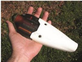
The *Acousonde™ 3B* is a self-contained underwater acoustic recorder comprising one or, optionally, two hydrophones, sensors for attitude, orientation, depth and temperature, a digital recorder, and a field-replaceable battery. Attached to an animal subject, the Acousonde measures the subject's sound environment and vocalization activity as well as potentially associated behavior.
