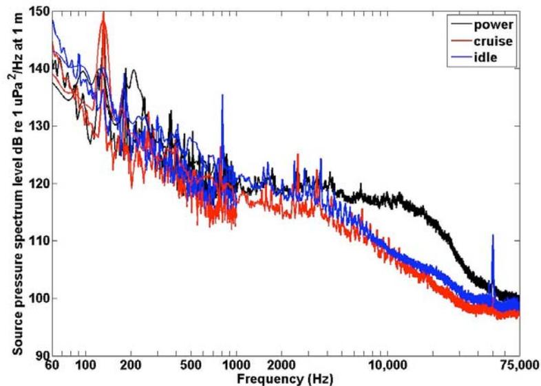
Figure 4. Annie Mae source spectral levels (dB re:  $\mu\text{Pa}^2/\text{Hz}$  @ 1 m). The spectral peak at 50 kHz in the idle data is an echosounder. The vertical array uppermost hydrophone is plotted to 1 kHz and overlaid by the broadband hydrophone data, which extends to 80 kHz. The power-up noise data at 8-30 kHz show as much as 10 dB increase over background noise levels.
