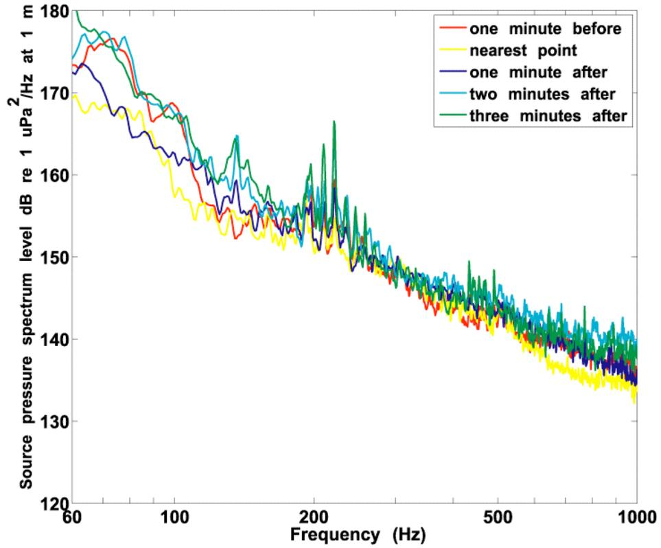
Figure 13. Computed source spectral levels (dB re:  $\mu\text{Pa}^2/\text{Hz}$  @ 1 m) of the Hanjin Marseilles are shown at various times as it passes our measurement site at a speed of 21 knots with a closest point of approach of 442 meters. Data are from channel one of the vertical array.
