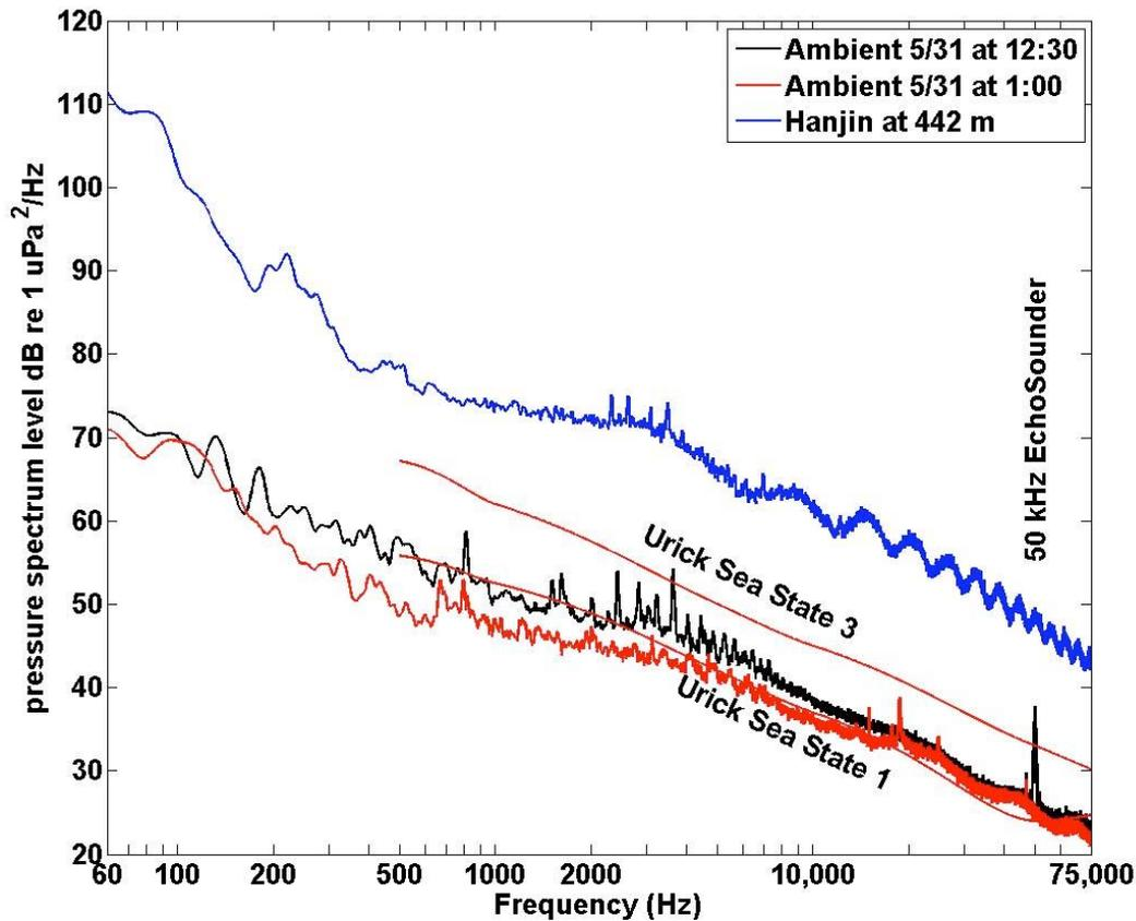
Figure 14. Received pressure spectrum level of the Hanjin Marseilles at 442 m compared to background ambient noise levels in sea state 2 at 12:30 increasing to sea state 3 at 1:00 and the deep water ambient levels of Urick (1983) for sea states 1 and 3.
