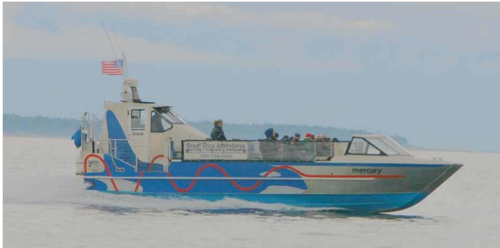
Figure 7. The Mercury is a 38' aluminum catamaran with jet drives.
