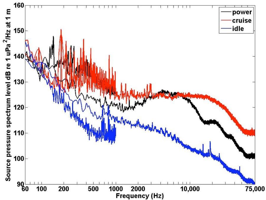
Figure 10. Olympus source spectral levels (dB re:  $\mu\text{Pa}^2/\text{Hz}$  @ 1 m). Vertical array data are plotted 60-1000 Hz and broadband hydrophone data from 60 – 75,000 Hz. The offsets at 1000 Hz between recordings systems may be related to slight time offsets in the two recording systems.
