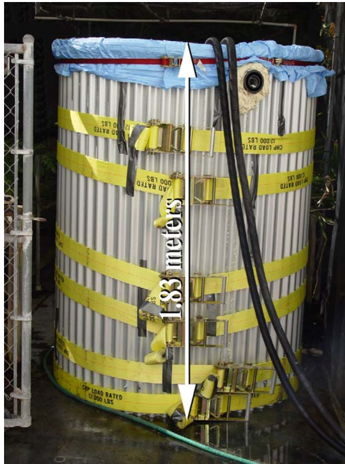
Figure 4.2: Portable reusable immersion tank. This chamber is used to thaw large frozen whale heads evenly and thoroughly so that they can be dissected. The cylindrical chamber is constructed of overlapping corrugated metal panels that hold a swimming pool liner and is retained with a series of nylon load straps. Between usages the chamber can be disassembled and stored in a relatively compact space.
