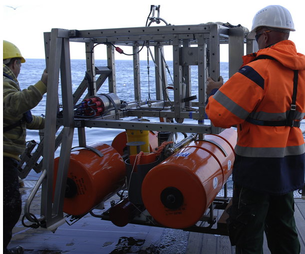
Figure 4. Photograph of Benthic Lander with HARP prior to deployment. Hydrophone is mounted horizontally above right-hand side orange tube toward the center of the lander, ADCP is yellow and pointing upward, and CTD is mounted horizontally to the frame (photograph by Peter Linke – GEOMAR). (For interpretation of the references to color in this figure legend, the reader is referred to the web version of this article.)
