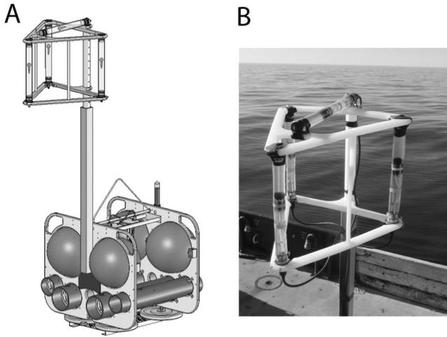
FIG. 3. (A) Schematic of tracking high-frequency acoustic recording package (THARP) with four-channel hydrophone array arranged in a tetrahedron configuration about 3 m above the seafloor. (B) Photo of tetrahedron array with sensors about 0.5 m apart.
