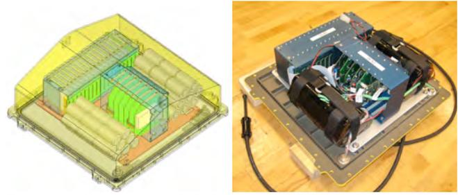
**Figure 3: Computer-aided design model and photo of HARP data logger integrated in a Wave Glider payload box.**
