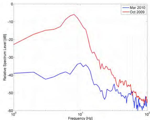
**Fig 7: Relative spectrum levels between 1 and 100 Hz for the October 2009 deployment with hard mounted cable (red) and for the March 2010 deployment using a cable fairing and flexible coupling (blue) show a reduction of low frequency self-noise of around 20-25 dB below 10 Hz.**
