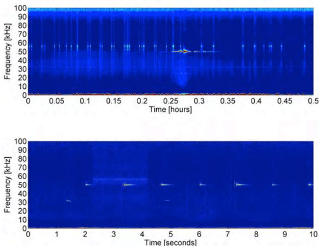
**Fig 5: Long duration (1/2 hr) spectrogram (top) and shorter duration (10 s) spectrogram (bottom) show 50 kHz echo sounder and broad-band, 2 second pulsed self-noise.**
