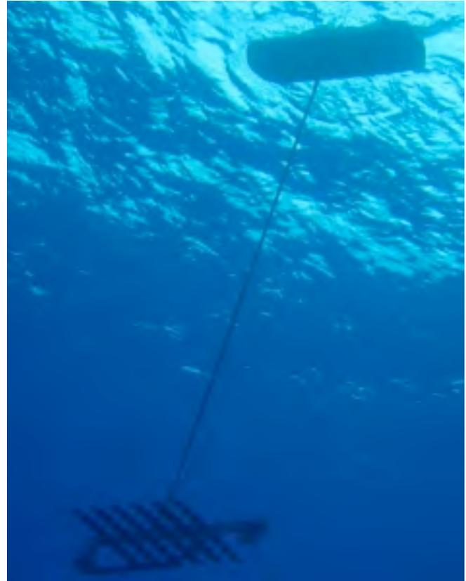
Figure 1: Wave Glider photo, showing the sea-surface vehicle tethered to the submerged glider by an electro-mechanical cable.
