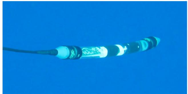
**Figure 4: Photo of the hydrophone and tow cable as it is towed behind the Wave Glider at sea.**
