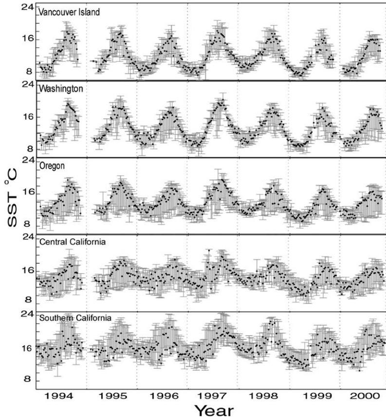
Fig. 5. Seven-day average SST values ( $^{\circ}\text{C}$ ) from each of the five geographic regions studied here from 1994 to 2000. Minimum and maximum values indicated by the gray bars. The El Niño of 1998 is seen as increased surface temperatures, particularly during the spring when upwelling usually lowers the surface temperatures substantially. Data available from: <ftp://podaac.jpl.nasa.gov/pub/seasurfacetemperature/avhrr/mcsst/data/weekly/day>.
